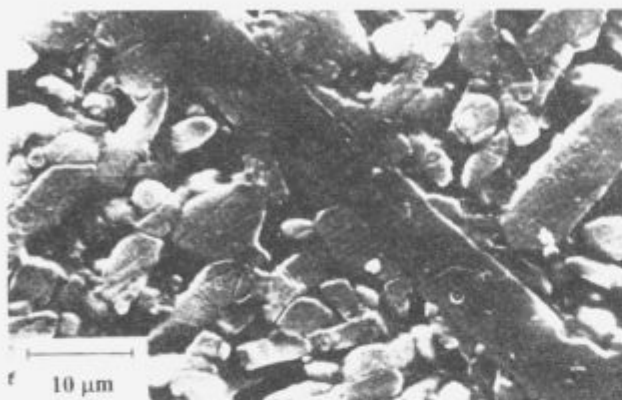
Figure 5: The polished and etched surface of B-Si 3 N 4 whisker reinforced \alpha -SiAlON (material R) Slika 5: Polirana in jedkana površina \alpha -SiAlON-a, utrjenega z B-Si 3 N 4 whiskerji. (material R)
