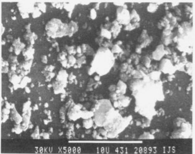
Slika 2: SEM posnetek RBAO prahu po mletju v acetonu Figure 2: SEM micrograph of RBAO powder after milling in acetone
