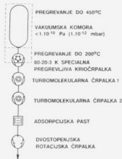
Slika 12: Shema EVV sistema z dvema turbomolekularnima črpalkama in tripanelno (80-20-3 K) specialno kriopumpo Figure 12: Schematic diagram of XHV system with two turbomolecular pumps and three-panel (80-20-3K) special cryopump
