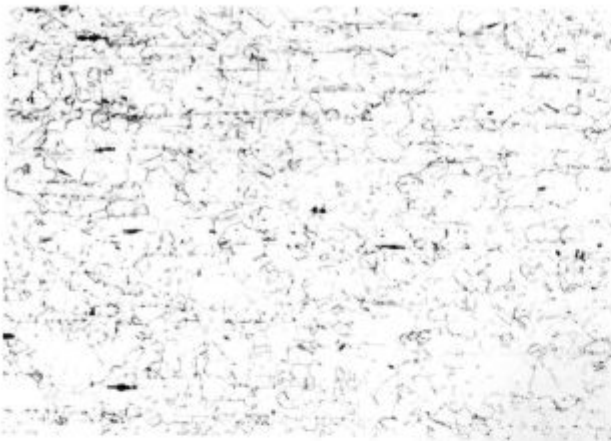
Slika 5: Mikrostruktura jekla 18/8 pred vlečenjem (povečava 100x) Figure 5: Microstructure of stainless steel 18/8 before drawing (100x)
