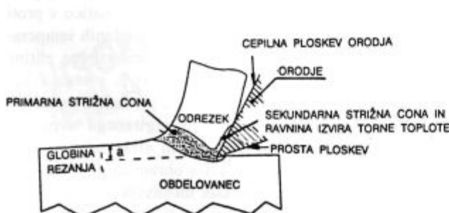
Slika 1: Razmere pri finem struženju v strižni coni Figure 1: Circumstances in fine turning in shear zone
