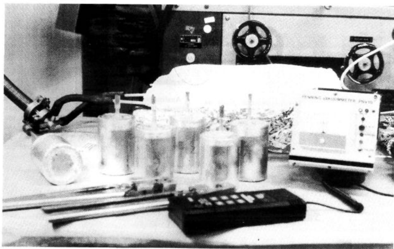
Slika 2: Evakuirane posode s CIP vzorci Figure 2: Evacuated container with the CIP samples
