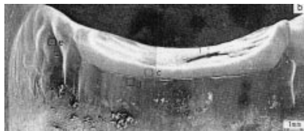
Slika 8: Krater obrabe na -lenu elevatorske verige Figure 8: Wear crater on elevator chain link
