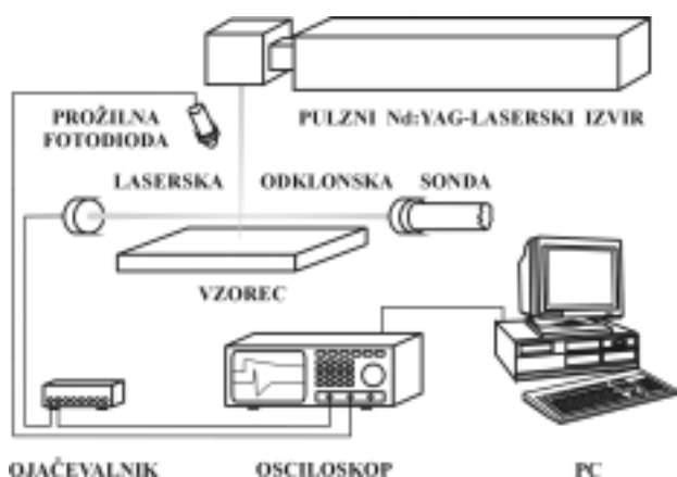
Slika 1: Shema eksperimenta Figure 1: Experimental set-up
