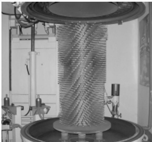
Slika 1: Način saržiranja batnic plinskih amortizerjev Figure 1: Load configuration of gas shock absorbers' piston rods
