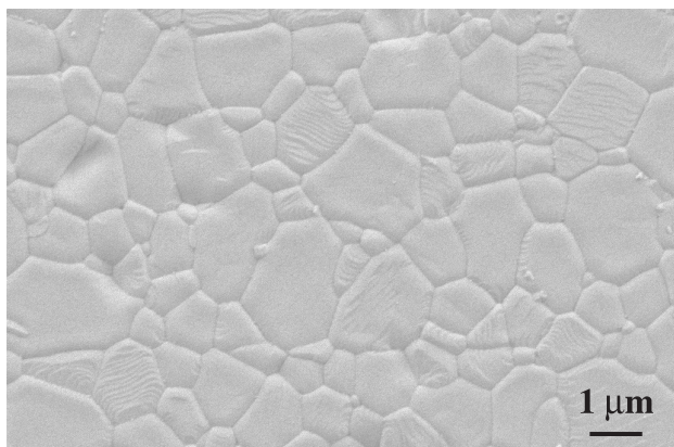
Figure 5: Microstructure of polished and thermally etched sample S1 after sintering at 1150 °C (the dense region)
