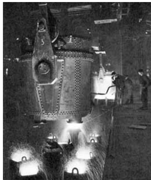
Figure 13: Casting in moulds Slika 13: Ulivanje kokil
