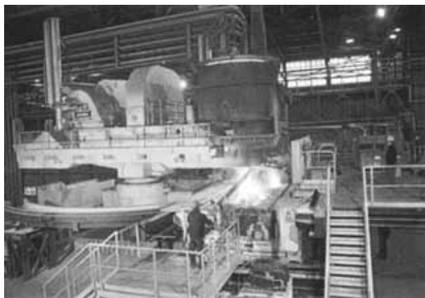
Figure 15: The new electric arc furnace 100 t Slika 15: Nova elektrobločna peč
