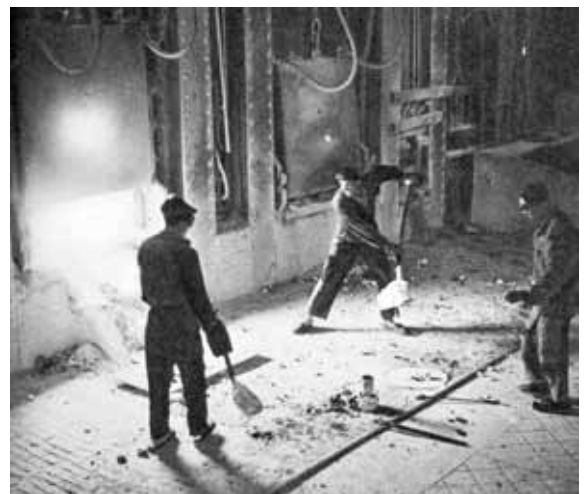
Figure 8: Manual charging of additions in the SM furnace
