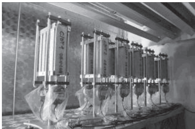
Figure 8: Apparatus for measuring an expansion of hardened concrete according to ASTM C490-86, placed in a climatic chamber
