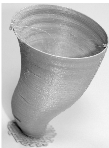
Figure 14: Thin-wall tornado (the wall thickness of only 0.55 mm) produced from LT3 PEEK
