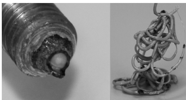
Figure 6: Degradation of PEEK inside the nozzle as a result of several heating cycles. The left figure shows the inside of the nozzle after being used for 15 cycles (15 working days). The right figure shows small particles that are caused by the material degradation inside the nozzle and are eventually deposited onto the product.
