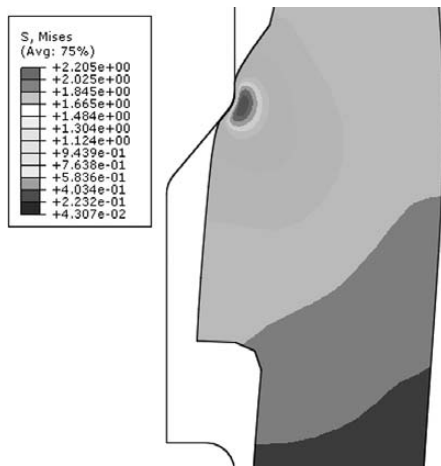
Figure 2: Stress field ( \beta = 40 mm, R = 10 mm, t = 3 mm)
