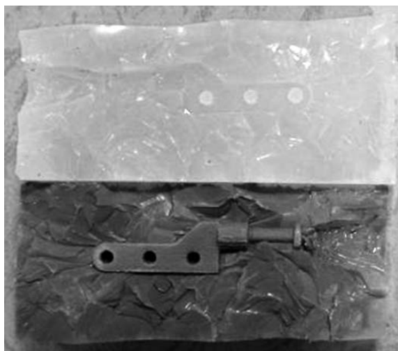
Figure 7: Green part of a male laptop hinge fabricated using a silicone rubber mold
