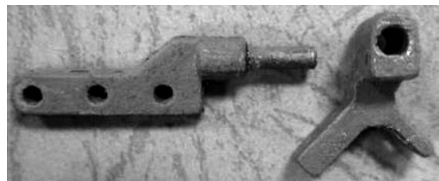
Figure 8: Metal prototypes of the laptop hinge after the post-curing process
