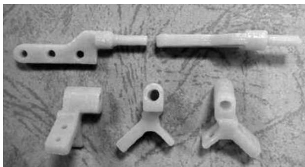
Figure 6: Wax patterns of the laptop hinge were replicated from the silicone rubber mold
