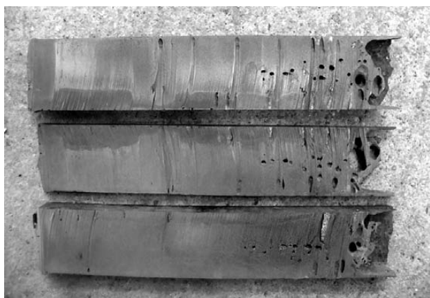
Figure 4: Longitudinal section of ingot cooled in iron mould. Gas bubbles and small closed shrinkage cavity moved toward the head. The solidification front moves toward the head, so the gas bubbles are concentrated below the head, where the last melt solidified.
