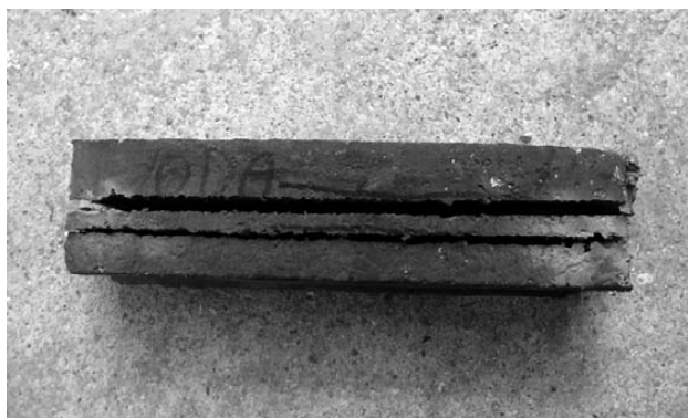
Figure 2: Longitudinal section of ingot cooled in water and cut with a high-pressure water jet cutter. The presence of gas bubbles disturbed the cutting process. The other two ingots were cut in the same way.
