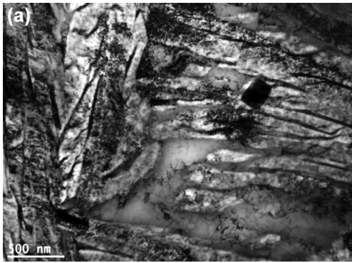
Figure 7: Block of retained austenite in the carburized surface layer on 35CrSiMn5-5-4 steel after austempering at 320 °C
