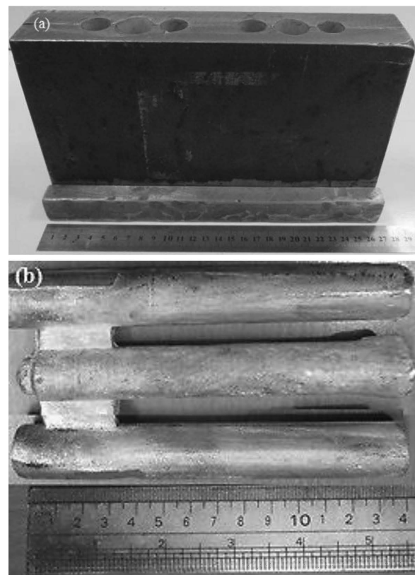
Figure 4: a) Steel mold used in this research, b) A cast sample in the mold
