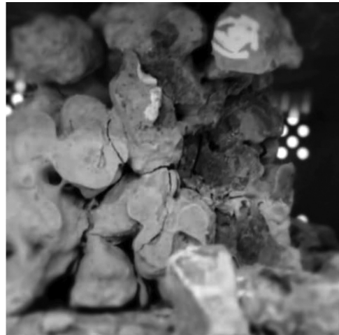
Figure 3: Compressive failure of a specimen
