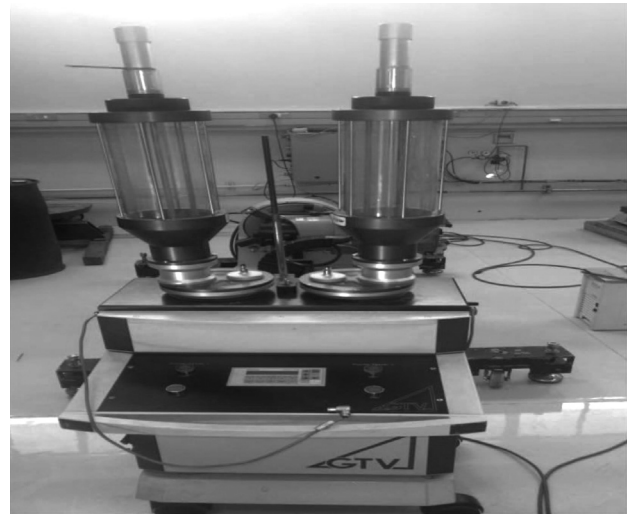
Figure 2: Double feeder of W and Ti6Al4V powders
