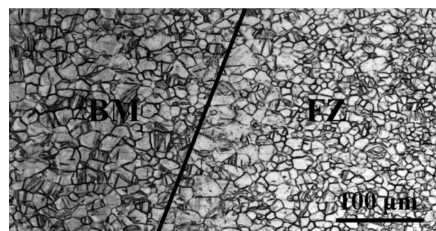
Figure 6: Top-surface microstructure of the AZ31B joint seam
