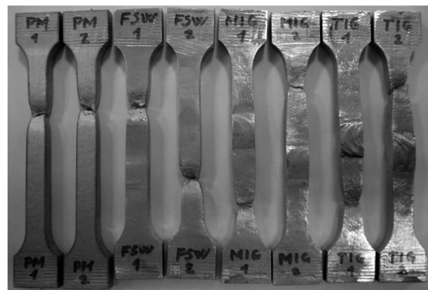
Figure 6: Specimen for tensile testing (1) and (2): PM – parent (base) material, FSW, MIG and TIG
