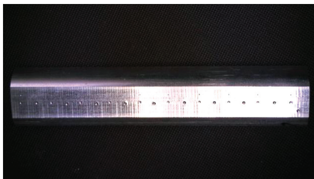
Figure 1: Examples of tested specimens with milled (left) and polished (right) surfaces
