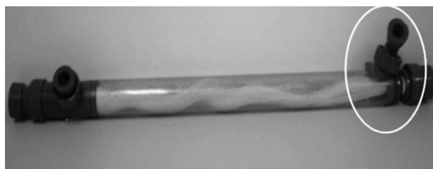
Figure 6: Shell-and-tube exchanger with a tangential inlet
