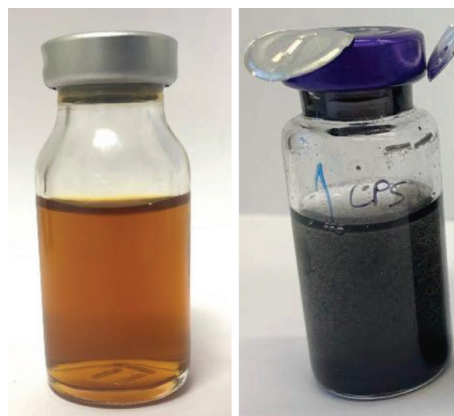
Figure 2: Control results of: a) IRB-bearing and b) SRB-bearing samples
